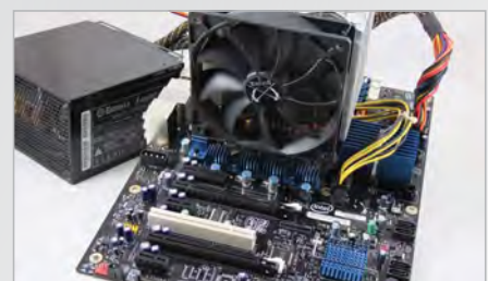
Take the case out of the equation to see if it's at fault
